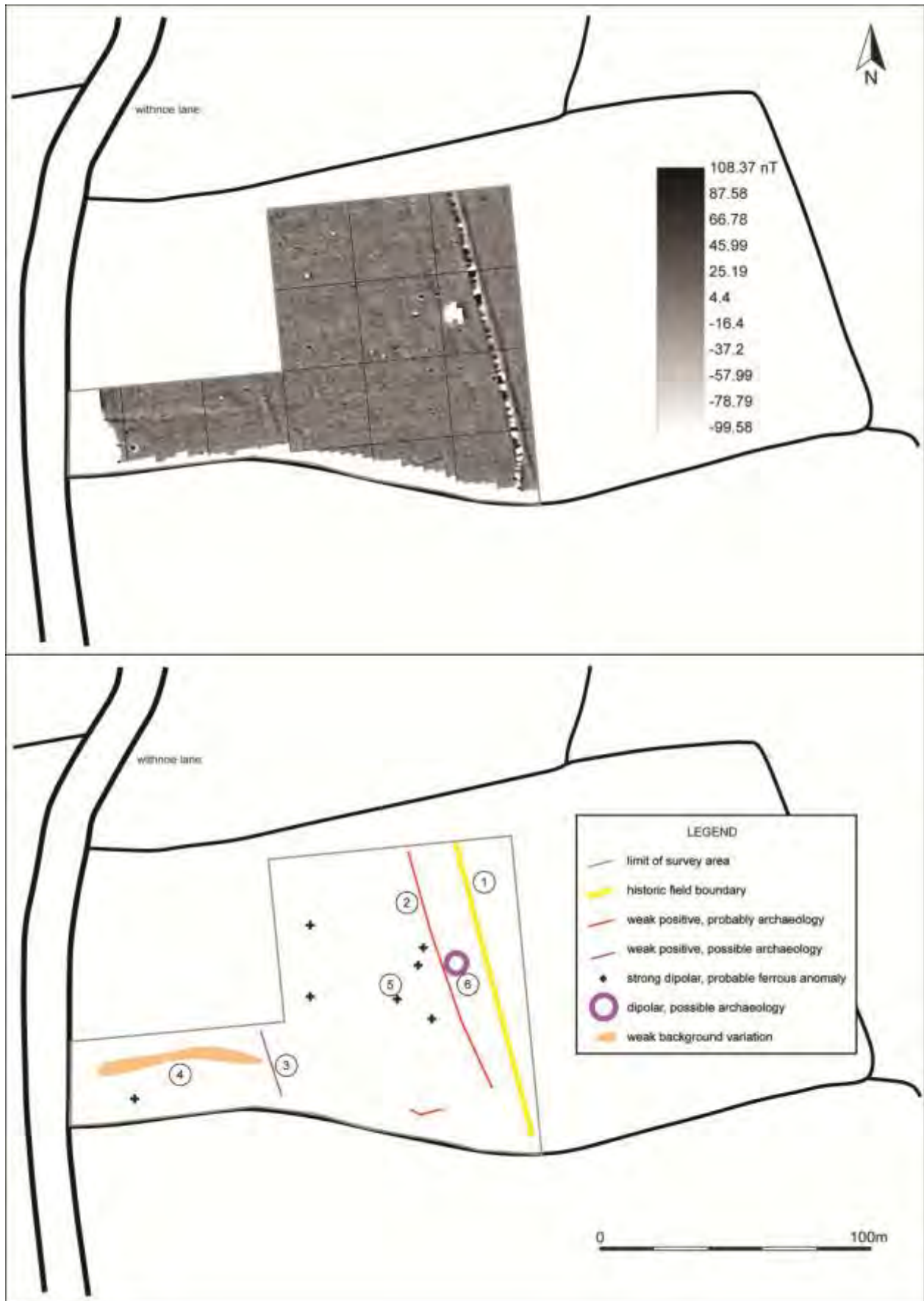
Figure 12: Above, shade plot of gradiometer survey data; below, interpretation of gradiometer survey data.
