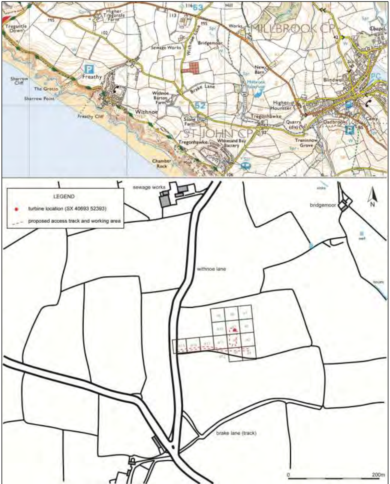
Proposed turbine location, location of geophysical survey grid, and respective numbers of survey grid squares.
